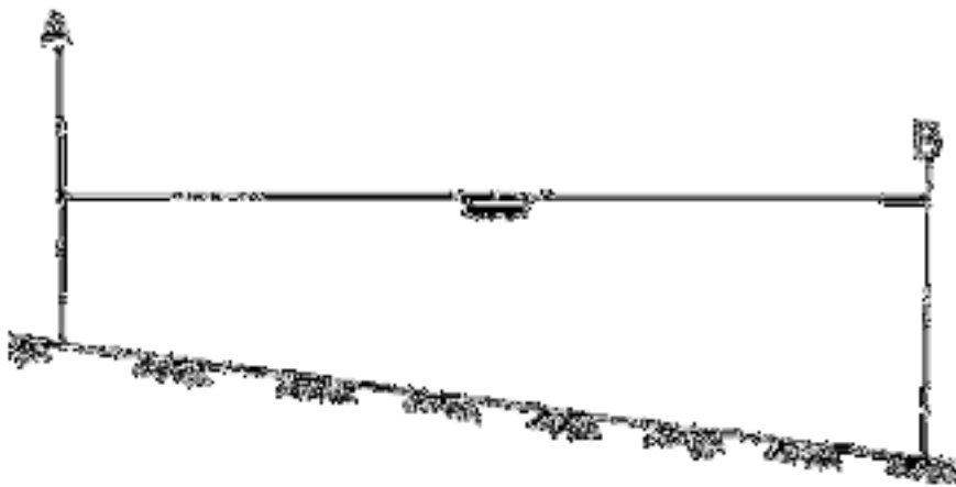
Figure 35. Measuring the slope with a line level
